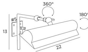
Classic painting lighting. Can be adjusted in depth through a set of two sliding tubes
